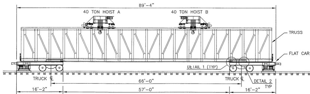
**Figure 4: Gantry Crane Profile**
