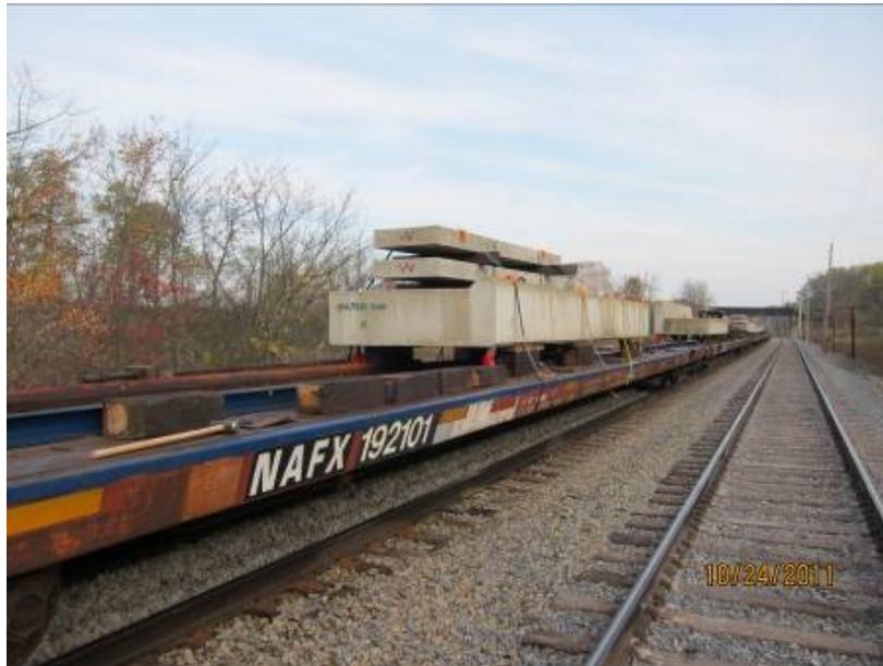
**Figure 7: Loaded Work Train Pre Change-out**
