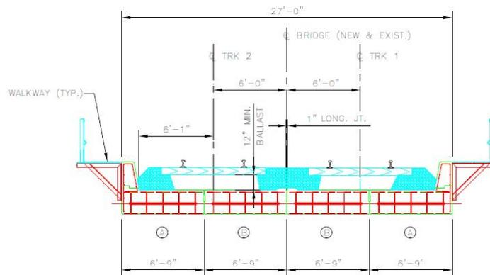
**Figure 3: Encased I-Beam Design Drawing**
